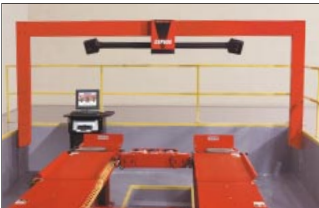
DSP600PM features overhead-mounted cameras for pit applications (shown with optional wall-mounted W cabinet).
